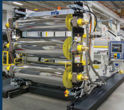
GCVD661824- A vertical down configured roll stand, ideal for medium gauge PP or PET.
