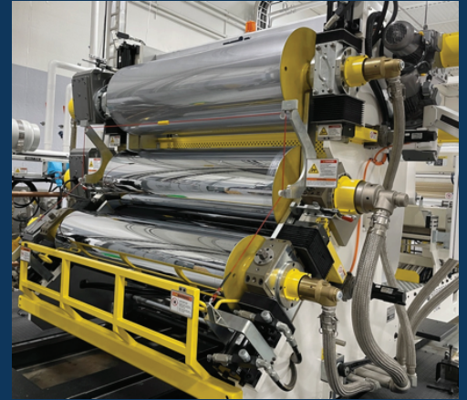
GCVD661830- A J-stack configuration, well suited for extended cooling requirements, low melt strength applications and thick sheet requirements.
